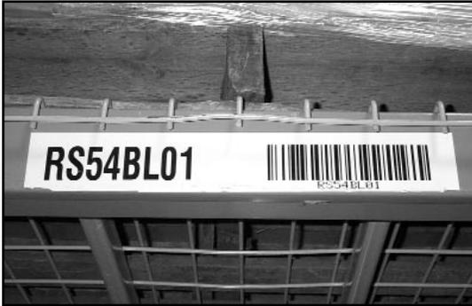
A warehouse operator transfers the material to an inventory location. These sites often are identified with bar codes printed on reflective labels. The reflective material (such as Zebra's RetroScan 4000 labels) improves readability from fork trucks up to 30 feet away. Bar codes are necessary because the operator scans both the package and the new storage location to complete the transfer operation and record it in the system.
